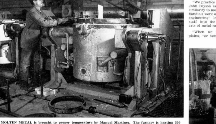
MOLTEN METAL is brought to proper temperature by Manuel Martinez. The furnace is heating 500 pounds of aluminum alloy to 1400 degrees fahrenheit. After the two-hour process is completed the crucible in the furnace is removed with a crane and taken to the mold.
